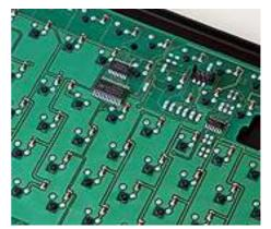
The seitches form the junction between the rows and the colums. As soon as a key is <u>Presse</u>d these paths are connected and tell the controller which key os pressed.
