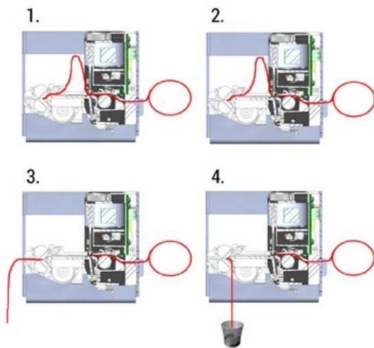
The loop-presenter (1.) transports the already printed paper, prior to Cut (2.) and paper output (3.), upward. Maximum paper thickness and ticket length need to be regarded, since loops can get to long and collapse or fall over and may cause a paper jam. Loop-Presenters can be offered with retract-function (4.).
