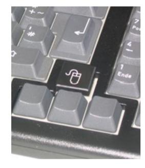
Due to the complete protection of the electronic components, all contacts and mechanic guide elements the long-travel keyboard is ideal for applications in rough environments.
