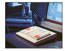
Degree of protection IP65 ensures that all contacts, electronic components and mechanical devices are protected from dust and water.
